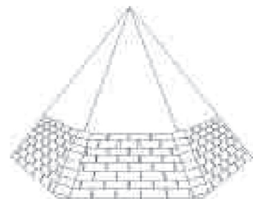
Figure 2 When roofing flat-sided cones, use the standard hip and ridge application method. Snap horizontal chalk lines to ensure a continuous roofing line.
